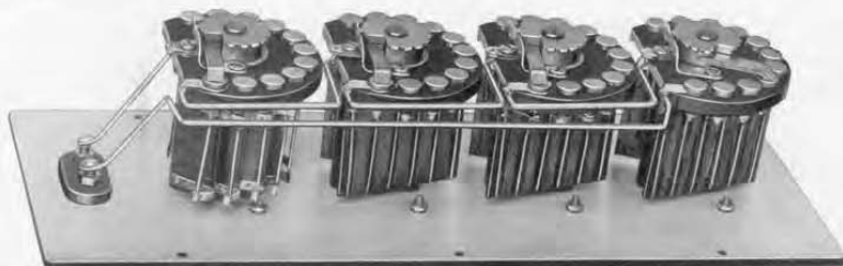
FIGURE 2. Interior of a TYPE 602-J Decade-Resistance Box. The decades are, from right to left, units, tens, hundreds, and thousands of ohms. A separate winding is used for each step
