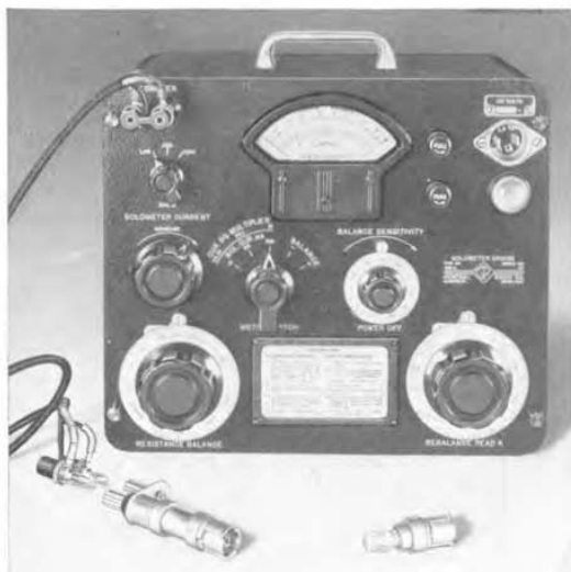
Figure 1. Panel view of the Type 1651-A Bolometer Bridge, with Type 874-H25 Thermistor Unit in left foreground.
