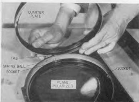
Figure 4. Quarter plate can be installed or removed without tools as shown here.
