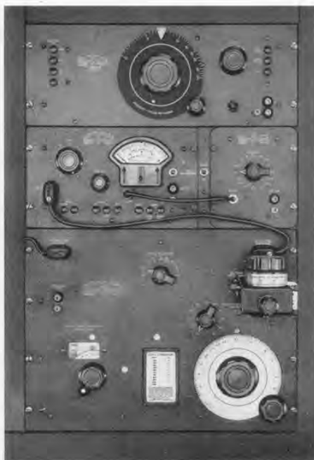
Figure 5. An assembly of equipment for dielectric measurements at frequencies between 50 cycles and 100 kilocycles, consisting of the Type 1302-A Oscillator, the Type 1231-BR Amplifier and Null Detector with Type 1231-P5R Filter, and the Type 716-C Capacitance Bridge, with the Type 1690-A Dielectric Sample Holder.
