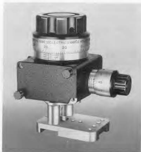
Figure 1. View of the Type 1690-A Dielectric Sample Holder.
