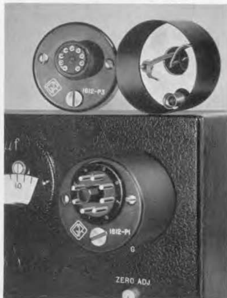
Figure 2. View showing the three socket adaptors, one attached to the X terminals of the capacitance meter. Internal view of adaptor at top right shows terminals, one of which is a lead for clamping in a binding post and the other a captive nut which replaces the binding-post cap.
