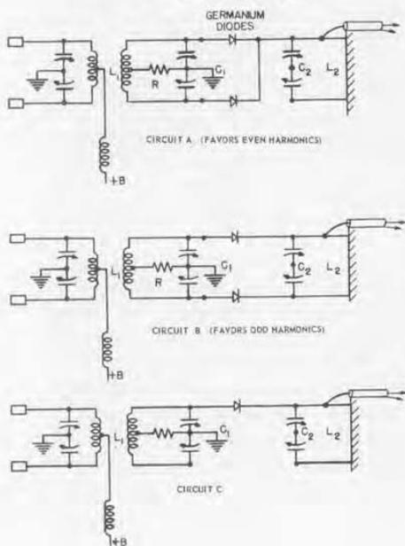
germanium crystal diodes operated as harmonic generators, as much as 60 milliwatts being available from a doubler stage at 500 Mc.
