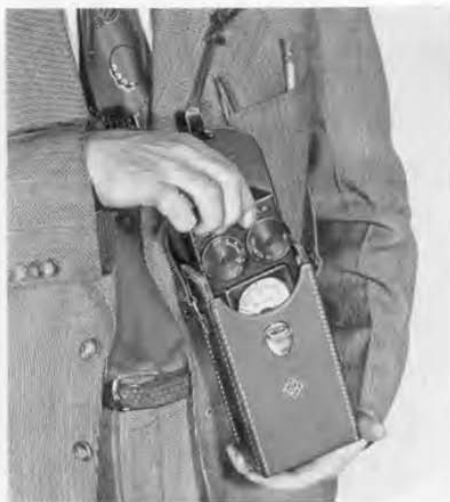
Figure 2. Convenient carrying case is made of brown, blister-proof, top-grain cowhide and has a shoulder strap. Space is provided for two spare flashlight cells and one spare plate battery.
