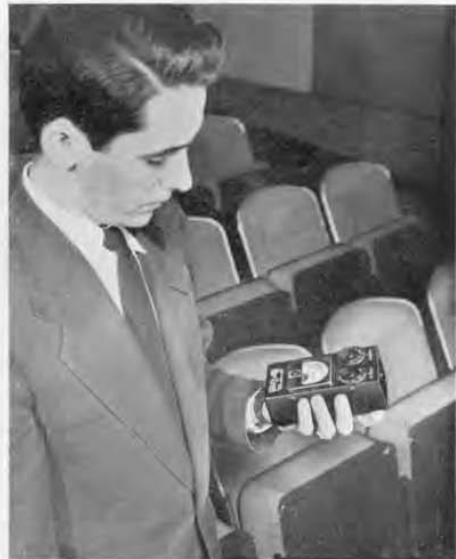
Figure 8. Measuring the level of reproduced sound in a theatre.
