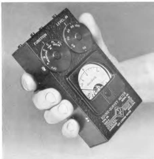
Figure 1. View of the Sound-Survey Meter, held in hand, with thumb in position to operate level control.
