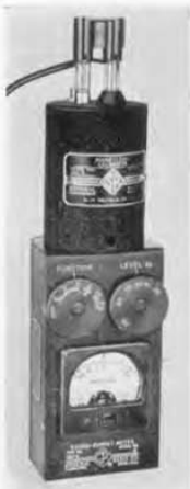
(Right) Figure 7. Sound-Survey Meter being used to measure noise level produced by pneumatic rock drills.
