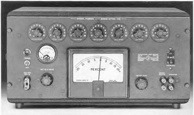
Figure 1. Panel view of the Type 1652-A Resistance Limit Bridge. Per cent deviation is indicated on the large meter, with its open, easily read scale.
