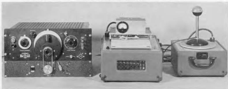
Figure 2. Complete assembly for measuring frequency response characteristics.
