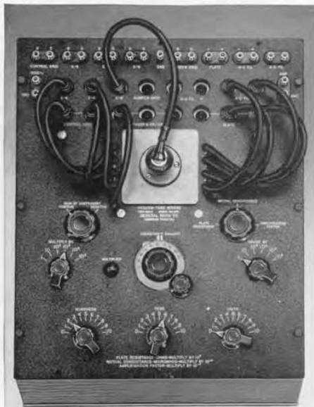
Figure 1. Panel view of the vacuum-tube bridge with adaptor and tube plugged into test position.
