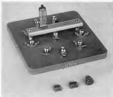
Figure 5 For sub-miniature types with short leads, sockets are supplied which can be mounted on the Universal adaptor. This photograph shows one way of mounting the Type SOT-50 7-pin socket (for flat-press tubes) on a Universal adaptor. In the foreground are shown, left to right, Type SOT-46 for 5-pin tubes, Type SOT-49 for 6-pin tubes, and Type SOT-48 for 8-wire sub-minar tubes.
