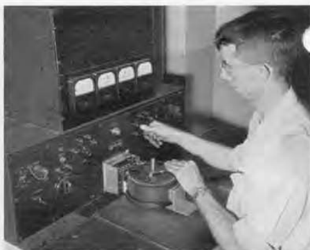
Prior to shipment, all Variacs must pass a series of rigid electrical tests to assure conformance to specifications.
