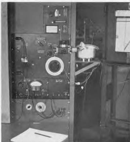
Figure 3. View of the measuring assembly at the Tennessee Eastman Company laboratories, showing the modified sample holder connected to a Type 716 Capacitance Bridge.
