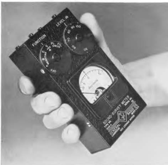
Figure 1. View of the Type 1555-A Sound-Survey Meter. When noise measurements are made with this instrument, the approximate frequency analysis is particularly useful.
