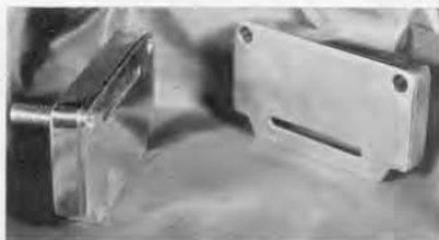
Figure 2. Close-up view of the covers, showing the slots through which air is pumped into, and exhausted from, the sample compartment.
