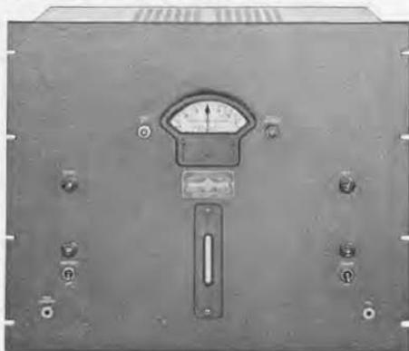
Figure 1. Panel view of the Type 1181-AT Color-Subcarrier Monitor.
