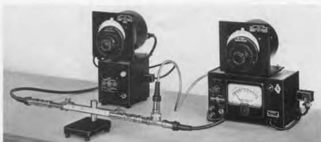
Figure 14. View of the Type DNT-1 Detector Assembly and a Type 1208-A Unit Oscillator set up for insertion-loss measurements on a 185-megacycle low-pass filter.
