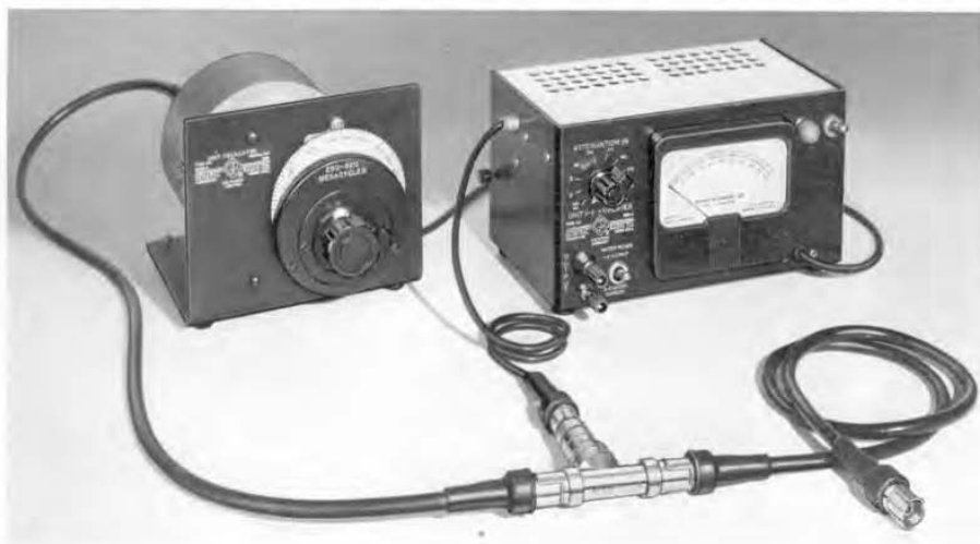
Figure 3. View of the DNT-3 Detector Assembly, utilizing General Radio coaxial elements and Unit Instruments.
