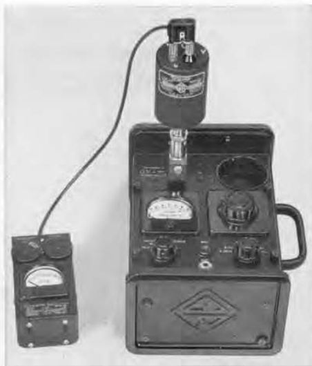
Figure 1. View of the Type 1552-B Sound-Level Calibrator, installed on the Type 1551-A Sound-Level Meter and driven by the Type 1307-A Transistor Oscillator.
