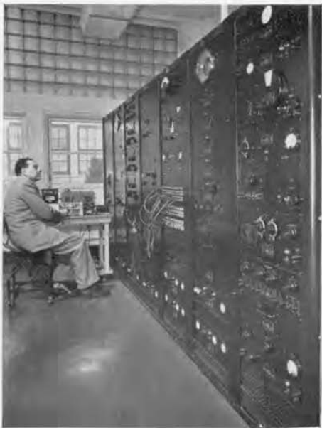
1955's Frequency Standardizing Equipment in the General Radio Engineering Laboratories.
