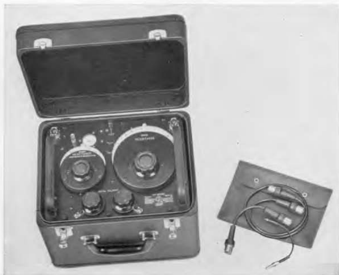
Figure 1. View of the Type 1606-A Radio-Frequency Bridge in its carrying case. Shielding is provided by the metal cabinet of the instrument, so that the bridge can be used either in or out of the carrying case.
