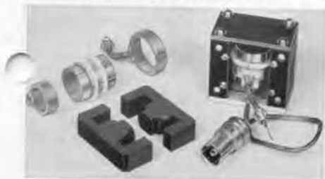
Figure 3. View of the bridge transformer with component parts shown at left.
