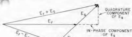
Figure 5. Phase-Sensitive Detector Operation.
