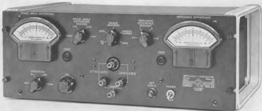
Figure 1. Panel View, Type 1605-A Impedance Comparator.
