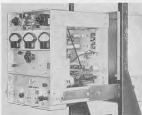
Figure 2. Front panel removes easily, and entire chassis pulls forward on slides for access to adjustments, test points, and tubes, with monitor operating.
