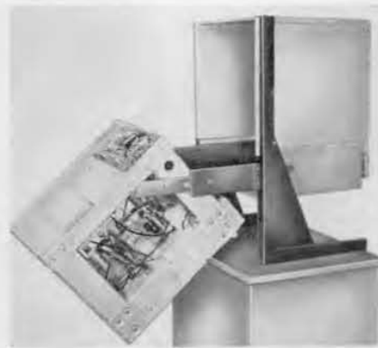
Figure 3. For access to rear or bottom, chassis tilts into this position and is held by latches. Monitor is still operating.
