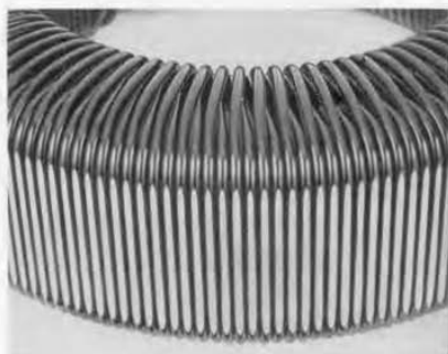
Figure 3. Close-up of the banked winding and Duratrak commutator surface.
