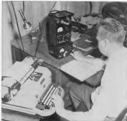
Figure 1. Setup used by Underwood for noise analyses of their "Golden Touch" typewriters. The transients are picked up by the suspended microphone, amplified by the Type 1551-A Sound-Level Meter, and then fed into the Type 1556-A Impact-Noise Analyzer.
