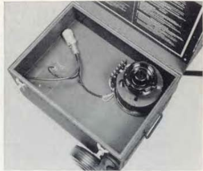
Figure 2. View of interior of Jetcal, showing the Type V-20 Variac ® Autotransformer in position.
