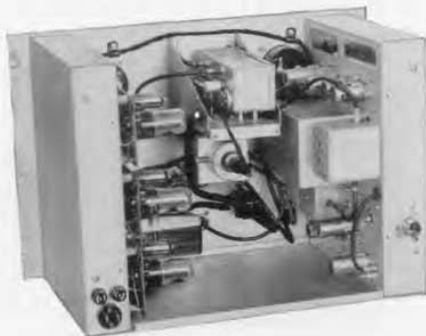
Figure 7. Rear view of Type 1112-B Standard Frequency Multiplier showing vertical chassis construction and r-f head (center).
