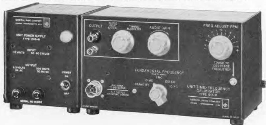
Figure 1. Panel view of the Type 1213-D Unit Time/Frequency Calibrator with Type 1203-B Unit Power Supply.
