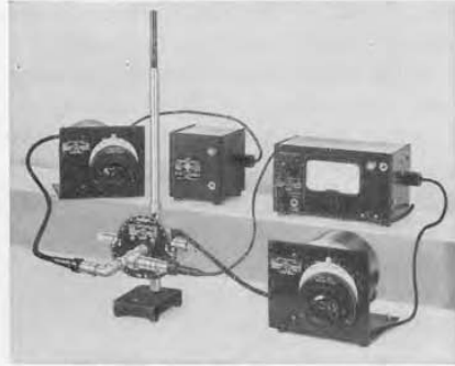
Figure 5. The Admittance Meter as set up for admittance or VSWR measurements, with a Type 1209-B Unit Oscillator and a Type DNT-3 Detector.
