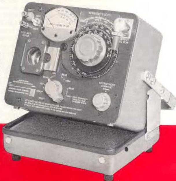
Figure 1. The Type 1559-A Microphone Reciprocity Calibrator is supplied in a Flip-Tilt case for convenient bench use. A relay-rack model is also available.
