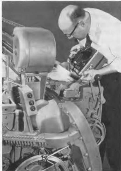
Figure 5. A typical application in the textile field: observing tape and filling-carrier behavior of a Draper DSL shuttleless loom. Speed of the filling carrier is 274 picks per minute. The Flash Delay makes it possible to observe the filling-carrier at any particular point on its path. Synchronization with loom is accomplished with the Type 1536-A Photoelectric Pickoff located near a rim connected to the main power shaft and shown at the bottom of the photograph.
