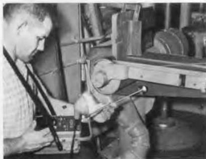
Figure 2. Measuring belt speed with the Surface-Speed Wheel.
