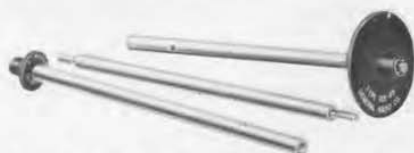
Figure 1. View of the Surface-Speed Wheel, showing the two speed discs and the sectional shaft.
