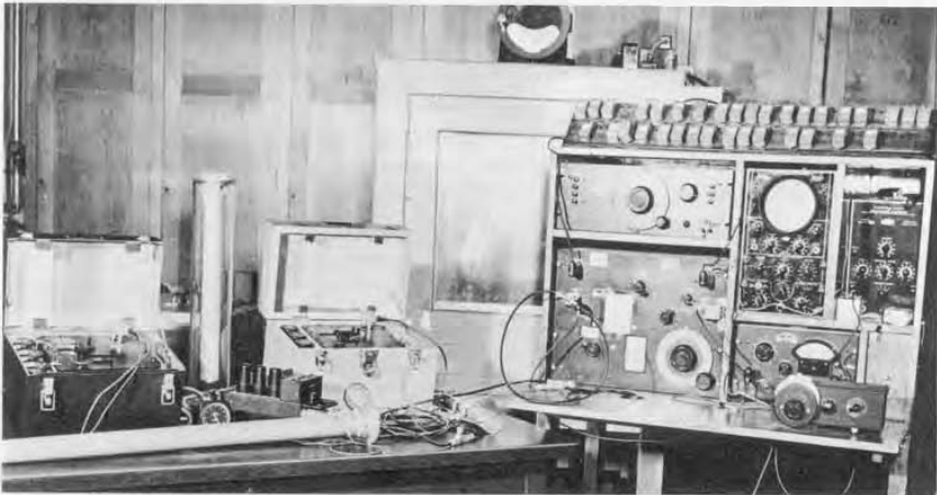
Equipment used in early fuel-gage tester development, shown in this 1951 photo taken at Aeronautical Instruments Laboratory, includes capacitance bridge, generator, and detector. (Official Photograph U. S. Navy)
