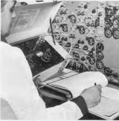
Technician calibrates fuel gage of modern jet aircraft by means of a GR Type 1429-A Fuel-Gage Tester.
