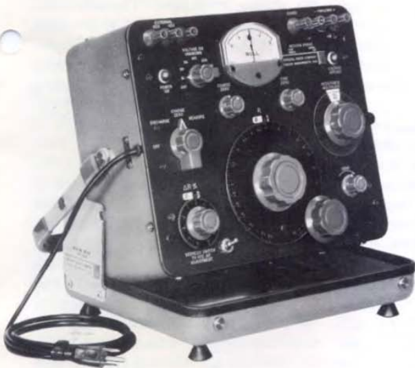
Figure 1. Panel view of the Type 1644-A Megohm Bridge. The Flip-Tilt case permits the panel to be positioned at any desired angle. Inset shows the older Type 544-B.
