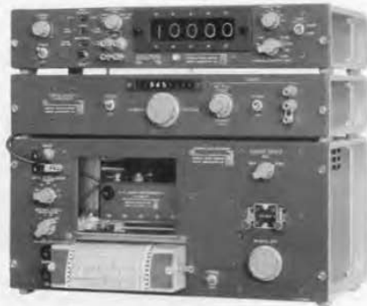
Figure 13. View of the Graphic Level Recorder bench-mounted with the Type 1151-AP Digital Time and Frequency Meter and the Type 1136-A Digital-to-Analog Converter.
