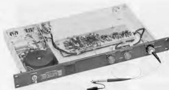
Figure 6. Tektronix oscilloscope probe (foreground) can be plugged directly into the scaler. The scaler input and output terminals can be mounted either on the panel or at the rear. Cover plates are provided for the panel when rear connections are used.
