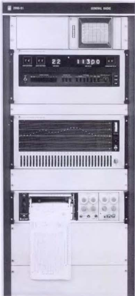
Figure 7a. Visual/record assembly including, from top to bottom, GR 1921-P1 Storage Display, GR 1926 Multichannel RMS Detector, GR 1925 Multifilter, and GR 1522 DC Recorder.
